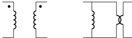
There is a fundamental difference between a transformer and two coupled inductors: in a transformer we wanted a very high magnetizing inductance, no matter its value; now, we want a **finite** and **controlled**  $L_p$  value (where  $L_p$  is again the magnetizing inductance, and “p” means **primary**, because we usually put it into the primary winding, even if it is not mandatory). Magnetizing inductance, in fact, is a model which represents the fact that this device can store energy!
