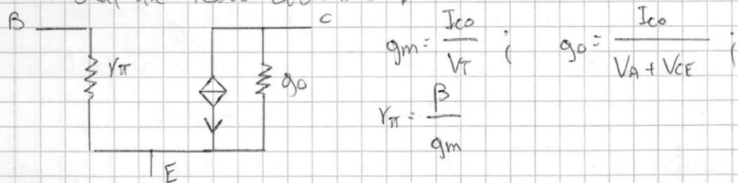
$$g_m = \frac{I_{CO}}{V_T} \quad ; \quad g_o = \frac{I_{CO}}{V_A + V_{CE}} \quad ; \quad r_{\pi} = \frac{\beta}{g_m}$$
