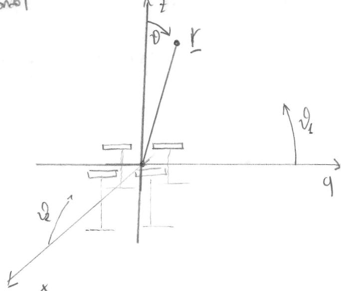
$$\hookrightarrow A(\vartheta, \varphi) = \sin(kh \cos \vartheta) \cos\left(\frac{Kd}{2} \sin \vartheta \cos \varphi\right) \cos\left(\frac{\pi}{2} \sin \vartheta \sin \varphi\right) \frac{F_0}{\sqrt{1 - \sin^2 \vartheta \sin^2 \varphi}}$$
