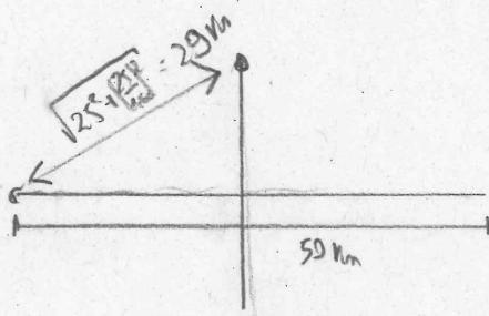
$$TX \rightarrow A = \sqrt{25^2 + \left(\frac{25}{1,66}\right)^2} = 29,2 \text{ Km}; \quad \text{arctan} \left(\frac{1}{1,66}\right) = 31,08^\circ$$
