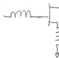
$$Z_{in} = \frac{V_{in}}{I_{in}} \rightarrow V_{in} = I_{in} \frac{1}{j\omega C} + I_{in} j\omega L \xrightarrow{\text{ign} \frac{I_{in}}{j\omega C}} j\omega L$$
