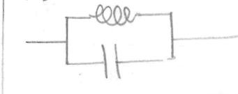
$$Z_{in} = \frac{L}{j\omega C_n - \frac{j}{\omega L_n}} ; \quad Y_P = \kappa^2 \frac{L}{j\omega L_S - \frac{j}{\omega C_S}}$$
