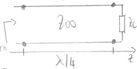
$$Z_{in} = \frac{Z_0^2}{Z_L} \quad \begin{array}{l} \text{noto da JRF parlando} \\ \text{di adattatore } \lambda/4 \end{array}$$
