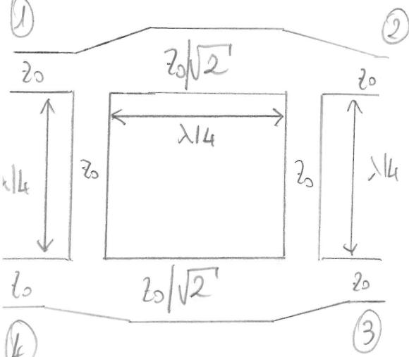
$$\underline{S} = \begin{bmatrix} S_{11} & S_{12} & S_{13} & S_{14} \\ S_{21} & S_{22} & S_{23} & S_{24} \\ S_{31} & S_{23} & S_{33} & S_{34} \\ S_{41} & S_{24} & S_{34} & S_{44} \end{bmatrix}$$
