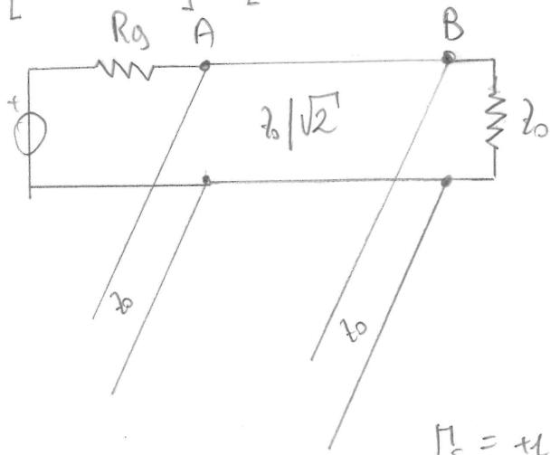
$$\begin{aligned} b_1^e &= \frac{V_A^-}{\sqrt{2}} ; b_2^e = \frac{V_B^+}{\sqrt{2}} ; \omega_0 = \omega_e = \frac{V_A^-}{\sqrt{2}\omega_0} \\ \frac{b_1^e}{\omega_0} &= \frac{V_A^-}{\sqrt{2}\omega_0} = \Gamma_{A-} ; \frac{b_2^e}{\omega_0} = \frac{V_B^+}{\sqrt{2}\omega_0} = \Gamma_{B+} \\ \end{aligned}$$
